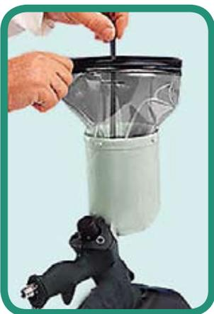
The amount of solvent needed to clean equipment can be greatly reduced by using disposable paint gun liners. Most of the solvent used for spray equipment cleaning is used to remove residual coating from the paint pot. If paint cup liners are used, the residual coating cures in the liner, and is disposed of. This eliminates the need to clean the paint pot. See the "Paint Waste Minimization Fact Sheet" for more information.
